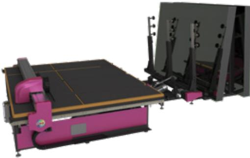
It is used for cutting straight and shaped or soft coated (Low-E) glasses. Thanks to the integrated loading arms, the glass sheet is automatically loaded from the glass stock stand.
